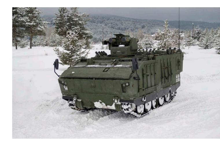
The hull of the KAPLAN-10 is manufactured and integrated using a ballistic welding technique. The power pack and driver are located in the front of the vehicle while the commander and gunner are situated in the centre. The rear part also hosts the gunner's aid and room for additional crew members.
